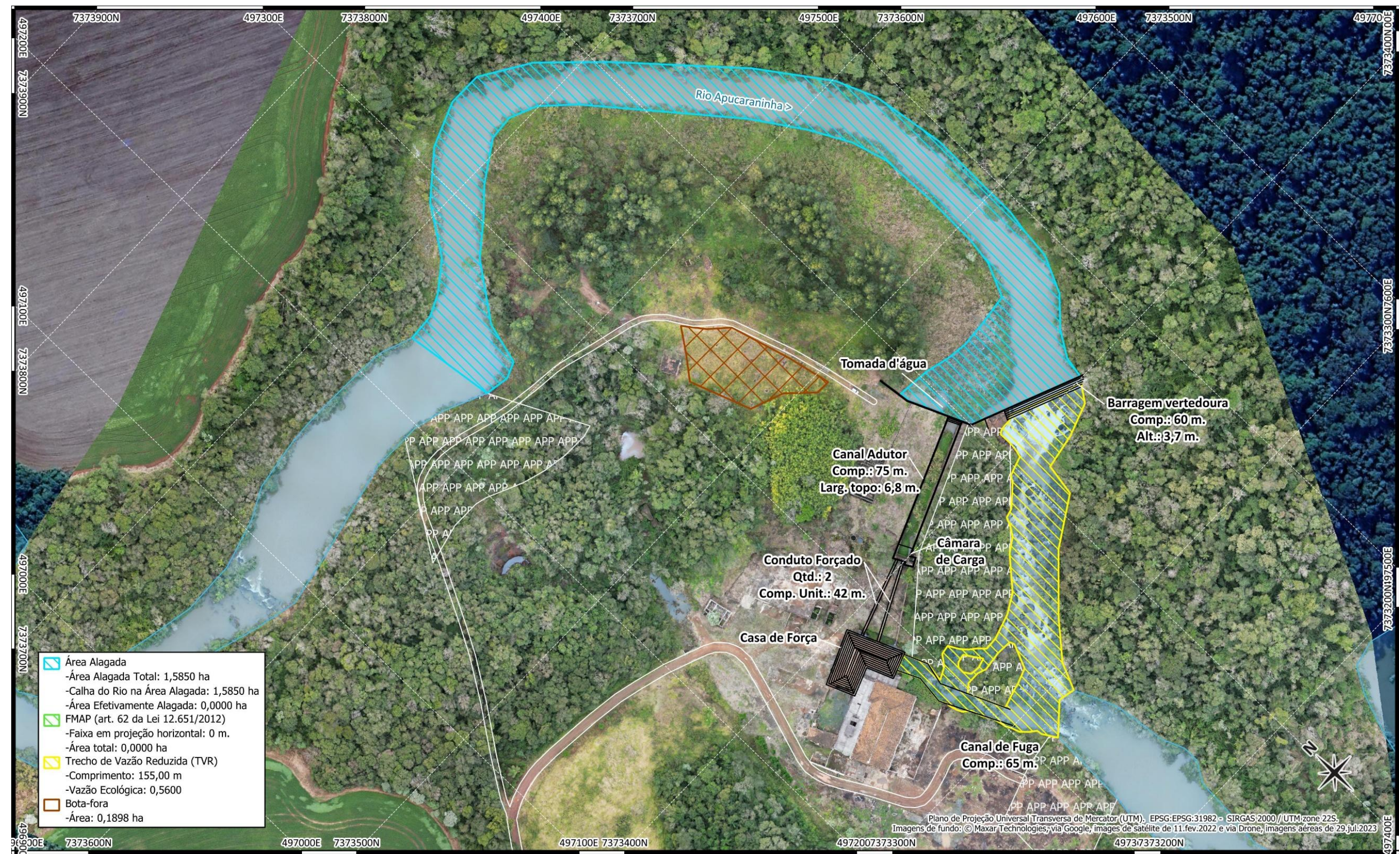
Figura 7- Arranjo Geral da CGH Tamarana (as built).
